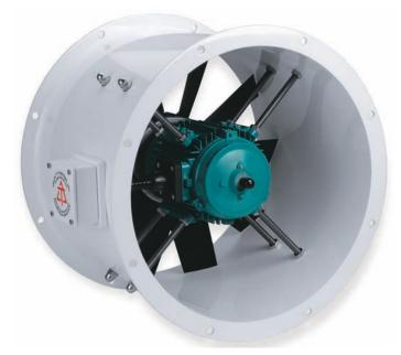
**Design & Construction** — Axial Ventilation Fans produced by Delta "T" Systems are specifically designed and built for the rigors of the marine environment — not adapted from other industries. Flanged housings of welded marine grade aluminum provide light weight and excellent corrosion resistance. Major assembly hardware is corrosion resistant stainless steel for long life. An external junction box mounted on the housing exterior is provided for electrical connections.
